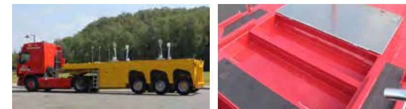
An integrated power-pack with batteries, charged while driving, for operating the trailer in all situations. Independent on every road.
