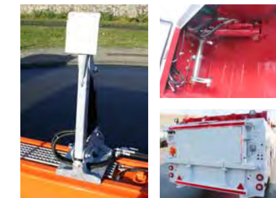
Hydraulic load-securing, covered rear door, vertical or combined opening of the rear door - there are many options for your Flatliner.
