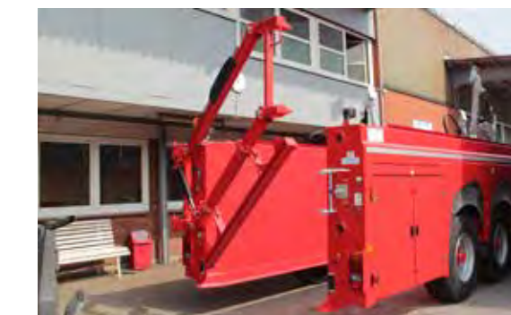
Hydraulic load-securing, covered rear door, vertical or combined opening of the rear door - there are many options for your Flatliner.
